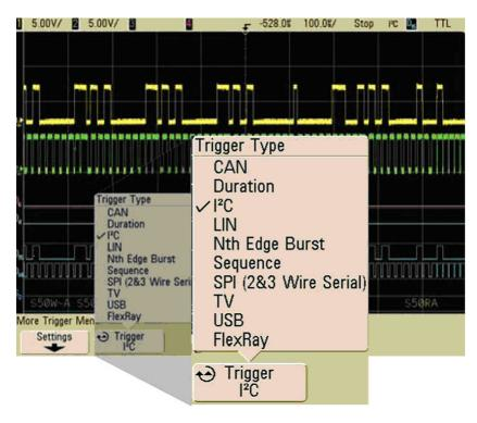
Figure 21. The Trigger Type menu appears when you push the softkey underneath the trigger menu.
