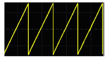
Figure 6. A sawtooth wave.
