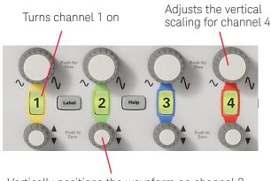
Vertically positions the waveform on channel 2
