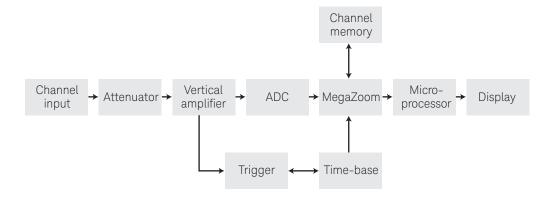
Figure 12. Digitizing oscilloscope architecture.
