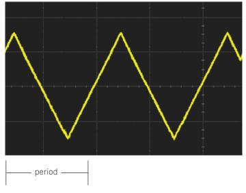
Figure 2. The period of a triangular wave.
