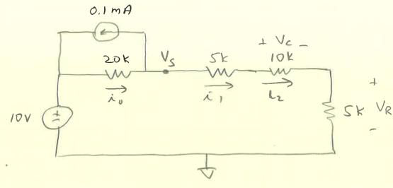
$$kcl @V_{S}: \frac{V_{S}-10}{20 \, K} + 0.1 \, m + \frac{V_{S}}{20 \, k} = 0$$
