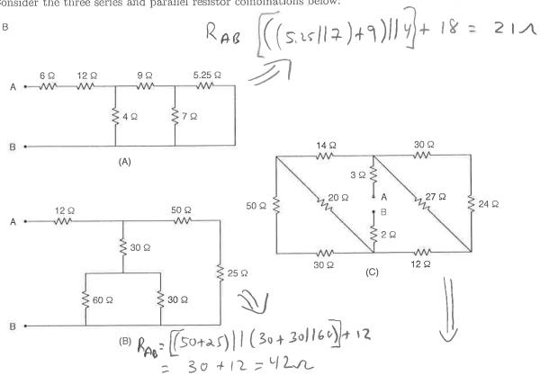
For circuits (A), (B), and (C) calculate  $R_{ab}$ , the equivalent resistance between terminals A and B:
