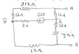
Part B: Draw the Thévenin Equivalent Circuit with respect to terminals A and B.
