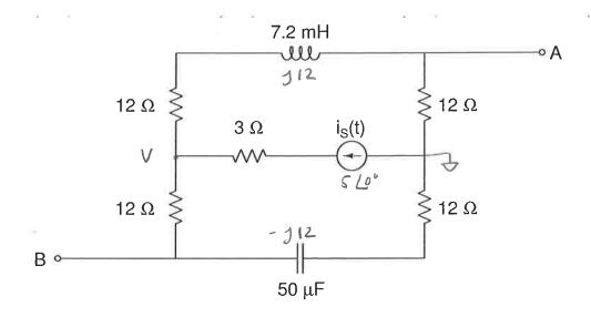
Part A: Draw the Phasor (frequency domain) representation of the circuit.
