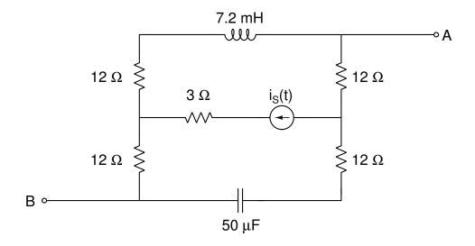
Part A: Draw the Phasor (frequency domain) representation of the circuit.
