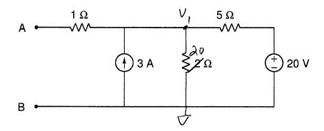
Part A: Draw the Thévenin Equivalent Circuit with respect to terminals A and B.
