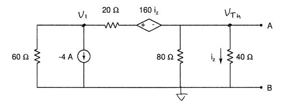
Draw the Thévenin Equivalent Circuit with respect to terminals A and B.
