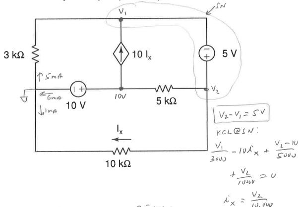
Power associated with the 5 V independent source? 25 mw
