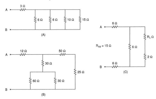
For circuits (A) and (B), calculate  $R_{ab}$ , the equivalent resistance between terminals A and B:
