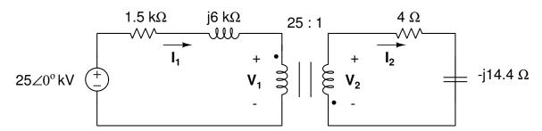
What is the Amplitude and Phase Angle of  $V_2$ ?
