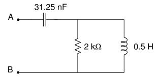
What is the equivalent impedance between terminals A and B?
