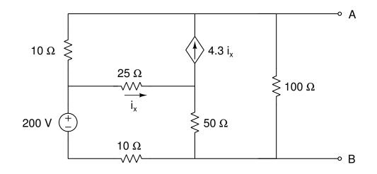
Part A: Draw the Thévenin Equivalent Circuit with respect to terminals A and B.
