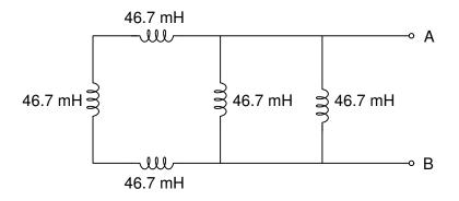
What is the equivalent inductance between terminals A and B?
