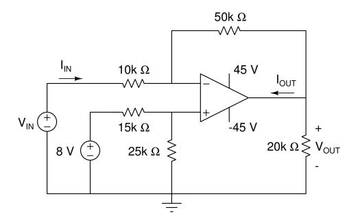
Derive an expression relating  $V_{OUT}$  as a function of  $V_{In}$ :
