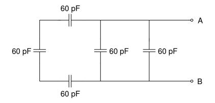
What is the equivalent capacitance between terminals A and B? \_\_\_\_\_
