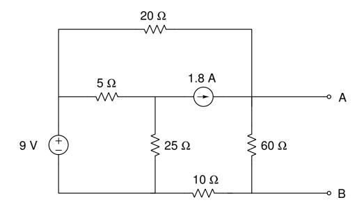
Part A: Draw the Thévenin Equivalent Circuit with respect to terminals A and B.
