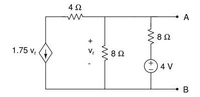
**Part A:** Draw the Thévenin equivalent circuit with respect to terminals A and B. Label the values of the circuit components.
