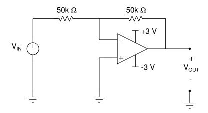
Derive an expression relating  $V_{OUT}$  as a function of  $V_{IN}\colon$  \_
