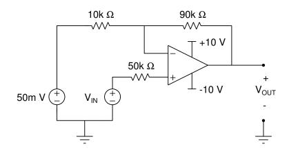
Derive an expression relating  $V_{OUT}$  as a function of  $V_{IN}$ :
