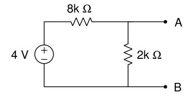
**Part A:** Draw the Thévenin equivalent circuit with respect to terminals A and B. Label the values of the circuit components.
