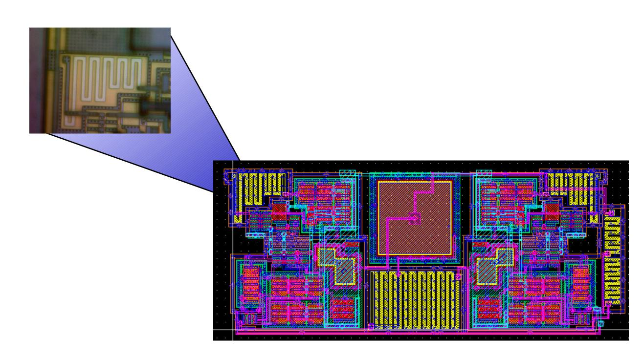
Microphotograph of 20k-ohm resistor (left) Layout view of wide-swing op-amp (right)
