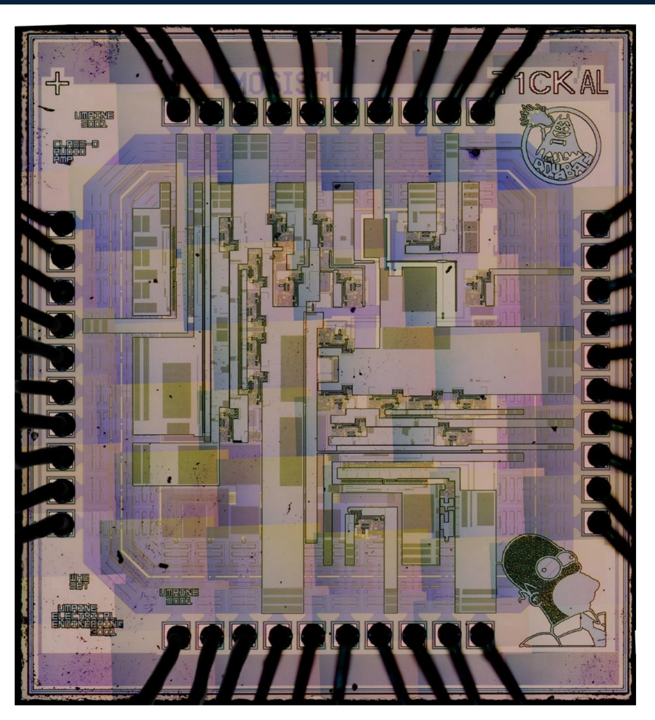
Microphotograph collage of circuit, 200x magnification (actual size 1.5 x 1.5 mm)
