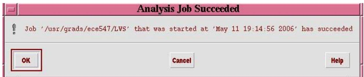
The Top-level layout of the circuit design does pass LVS.
