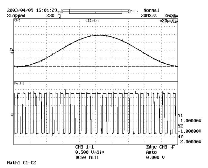
Figure 6.1 – PWM Test Waveform
