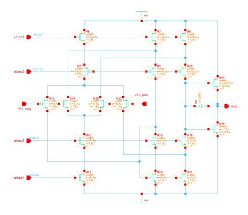
Figure A.5 – Wide Swing Op-Amp Gain Stage Schematic
