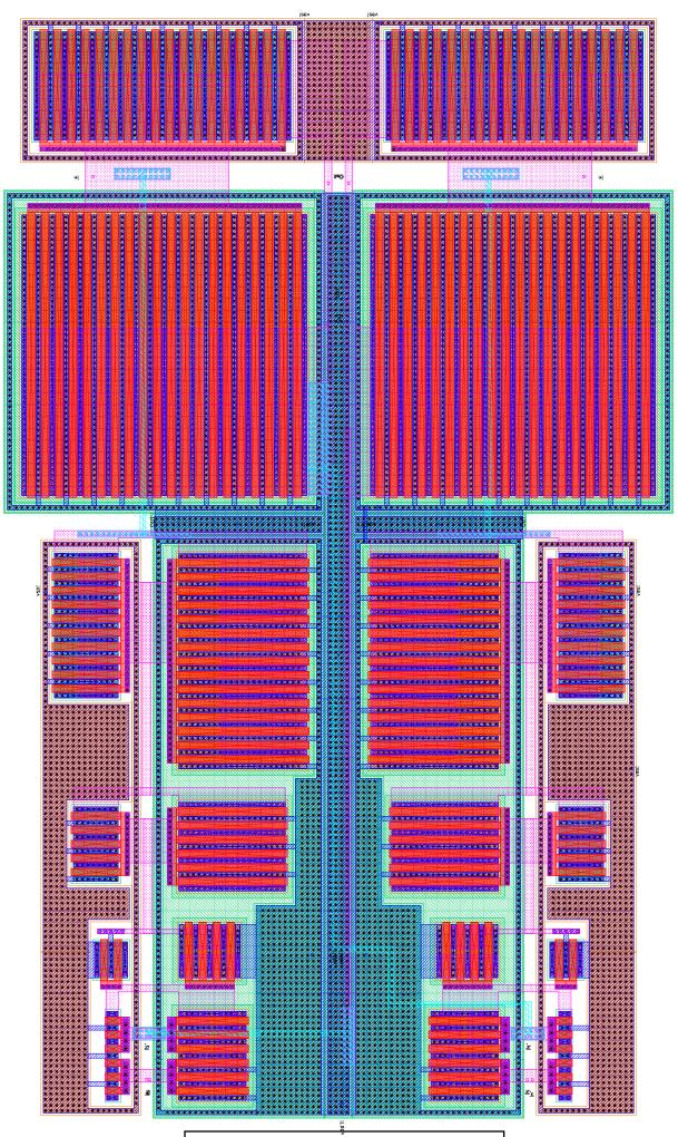
Figure B.11 -- H-Bridge Delay Layout
