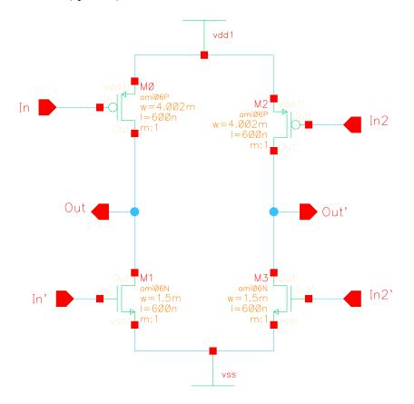
**Figure 2.14 – H-Bridge Schematic**
