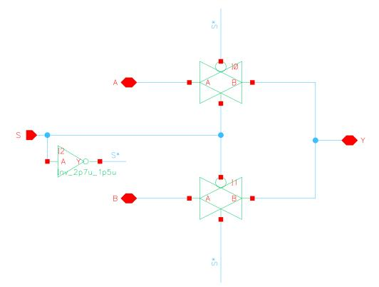
Figure A.6 – 2 to 1 Multiplexer Schematic
