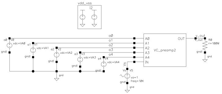
Figure 3.9 – Volume Control Preamplifier Test Circuit
