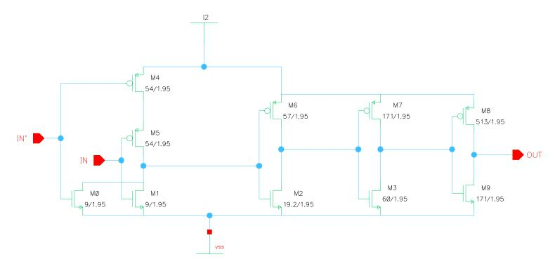
Figure A.15 – H-Bridge Delay Schematic
