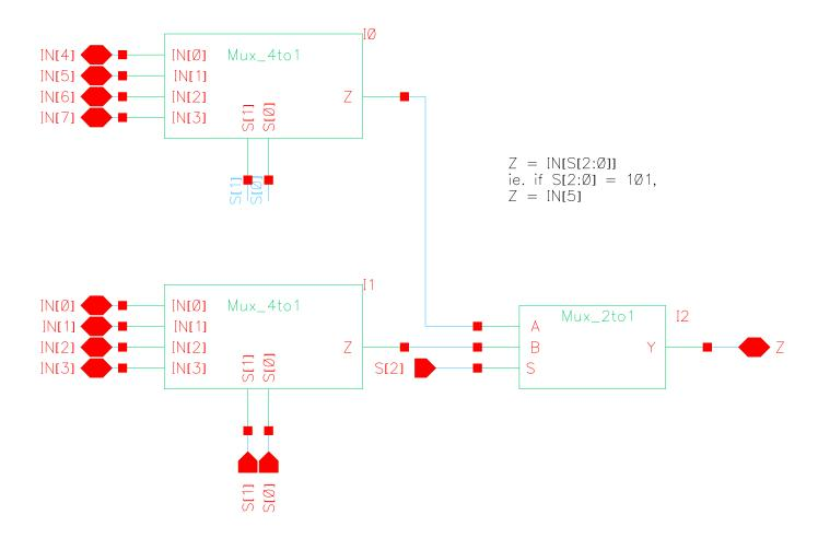
Figure A.8 – 8 to 1 Multiplexer Schematic
