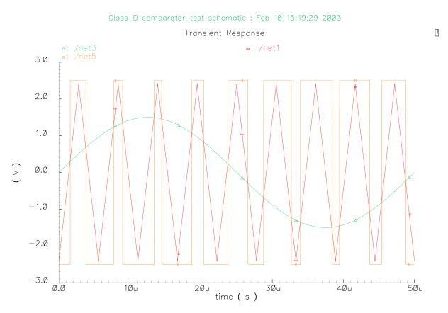
Figure 3.12 - Comparator (PWM) Test Waveform
