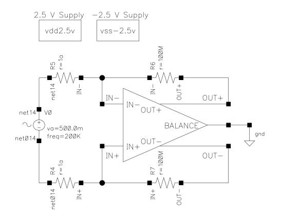
Figure 3.1 – Fully Differential Operational Amplifier AC Test Circuit
