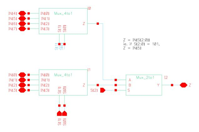
**Figure 2.4 – 8 to 1 Multiplexer Schematic**
