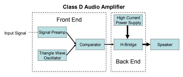
Figure 1.1 – Class-D Block Diagram
