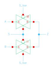
**Figure 2.2 – Transmission Gate Schematic**
