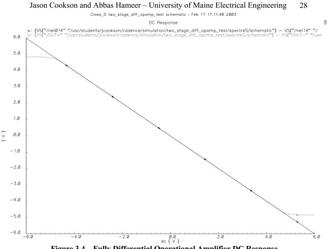
**Figure 3.4 – Fully Differential Operational Amplifier DC Response**
