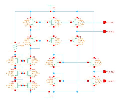
Figure A.4 – Wide Swing Op-Amp Bias Stage Schematic
