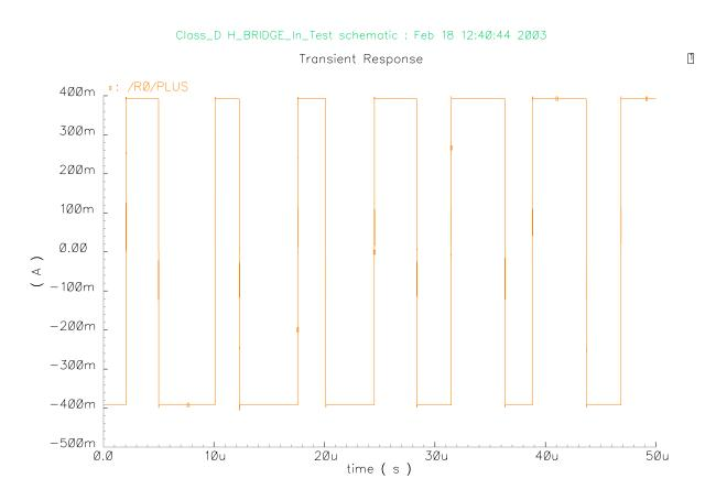
Figure 3.15 – H-Bridge Waveform
