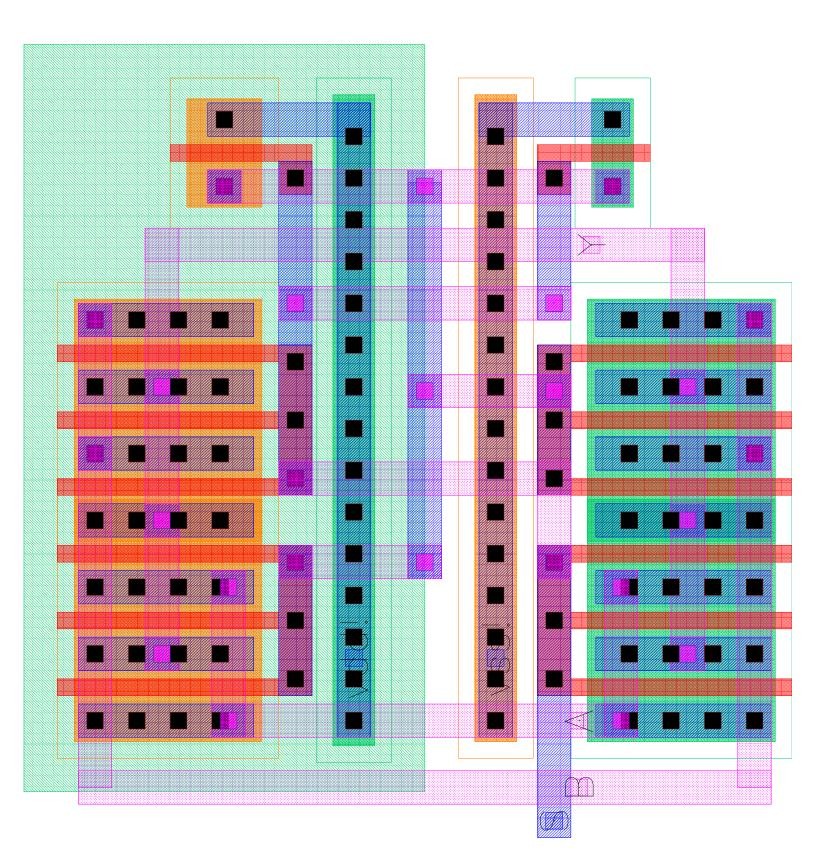
Figure B.3 -- 2 to 1 Multiplexer Layout
