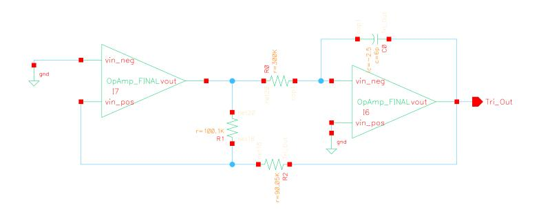
Figure A.13 – Triangle Wave Generator Schematic
