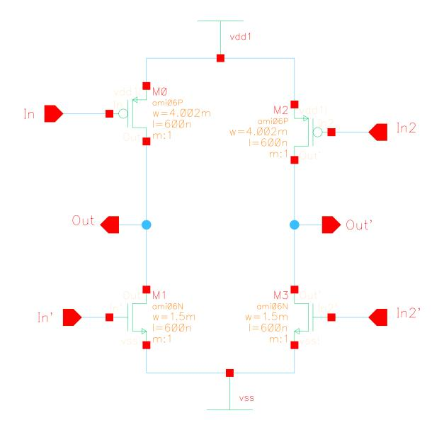
Figure A.16 – H-Bridge Schematic
