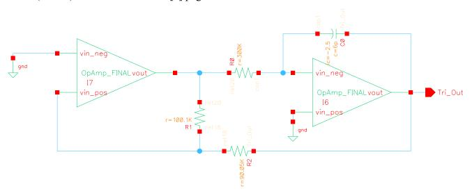
Figure 2.11 – Bi-Stable Oscillator Schematic
