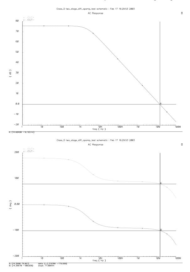
Figure 3.2 – Fully Differential Operational Amplifier AC Response
