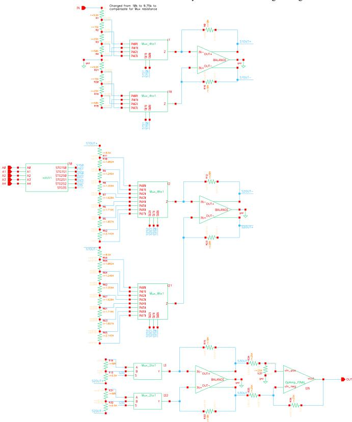
Figure A.12 – Volume Control Preamp Schematic
