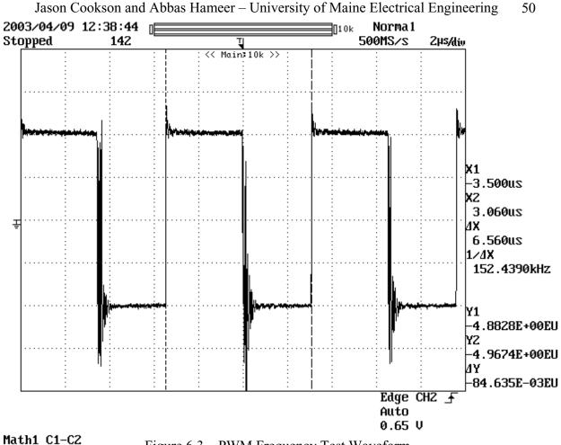
Figure 6.3 – PWM Frequency Test Waveform
