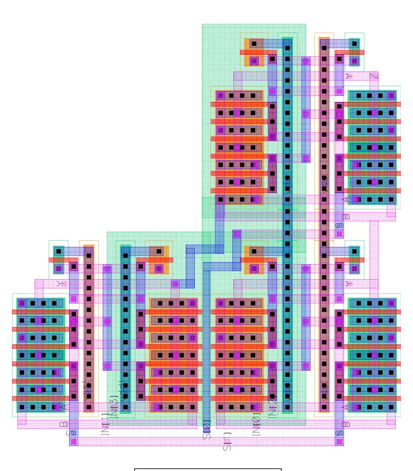
Figure B.4 -- 4 to 1 Multiplexer Layout
