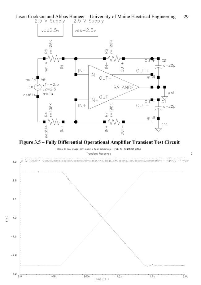
Figure 3.6 – Fully Differential Operational Amplifier Transient Response
