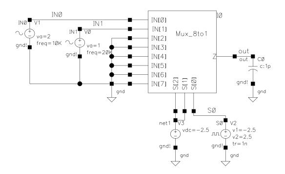
Figure 3.7 – 8 to 1 Multiplexer Test Circuit
