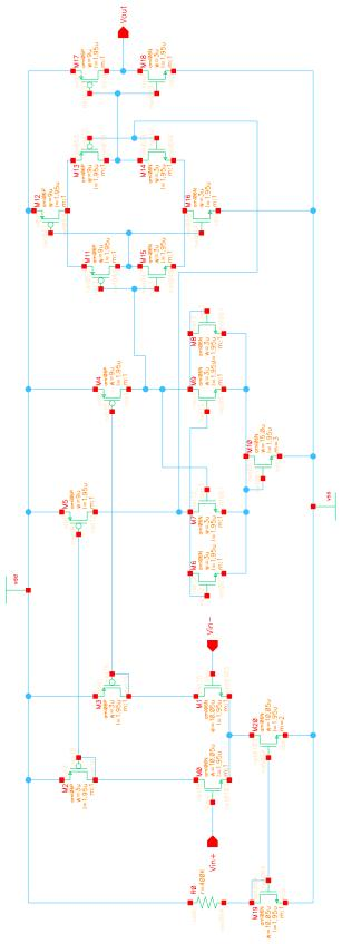
Figure A.14 – Comparator Schematic
