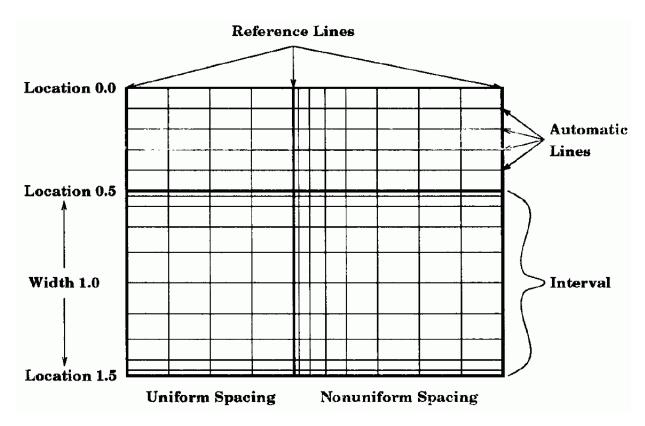
Figure 30.3: Typical mesh for 2D devices
