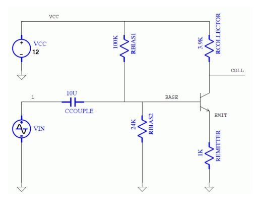
Figure 21.1: Transistor Amplifier Simulation Example
