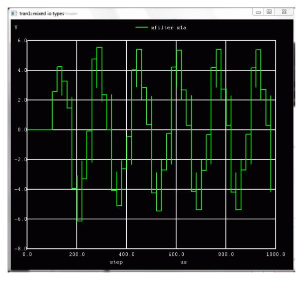
Figure 27.2: Nutmeg Plot of Filter Input and Output
