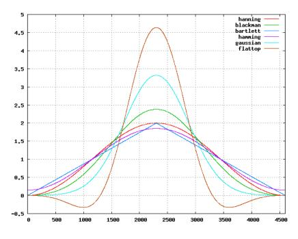
Figure 17.1: Spec and FFT window functions (Gaussian order = 4)
