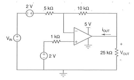
What type of circuit is this? Circle one: inverting amplifier, inverting amplifier with DC offset, noninverting amplifier, noninverting amplifier with DC offset, differentiator, integrator, Schmitt trigger.
