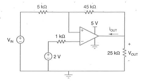
What type of circuit is this? Circle one: inverting amplifier, inverting amplifier with DC offset, noninverting amplifier, noninverting amplifier with DC offset, differentiator, integrator, Schmitt trigger.
